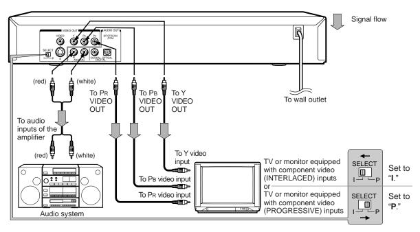
Switching the output signal (interlaced/ progressive) using the remote control (only when the SELECT (I/P) switch is set to "P")
